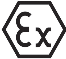
ATEX Approval for Zone 1 II 2G Ex ib IIB T4 Gb
